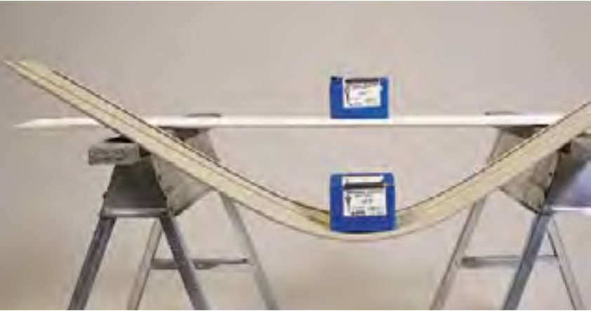
A COMPETITOR'S VINYL SIDING BENDS UNDER THE WEIGHT OF A TEN POUND BOX OF NAILS. POLAR WALL® PLUS! DOESN'T. IT'S AN EXTERIOR SYSTEM THAT'S EXTRA STRONG AND RIGID SO IT LAYS FLAT AGAINST THE WALL, RESISTS DENTS, WON'T BUCKLE, AND STAYS IN PLACE EVEN IN HIGH WINDS. TESTING PERFORMED WITH A DOUBLE 4" AND DOUBLE 5" DUTCHLAP PANEL.
