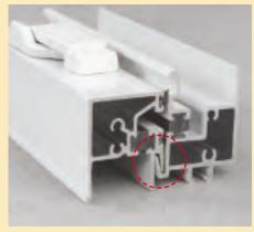
Interlock system locks both sashes together to prevent high winds from separating sashes, provides tighter seal and added security.
